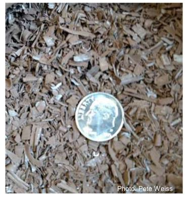
Connelly-GPM Iron Aggregate ETI CC-1004
