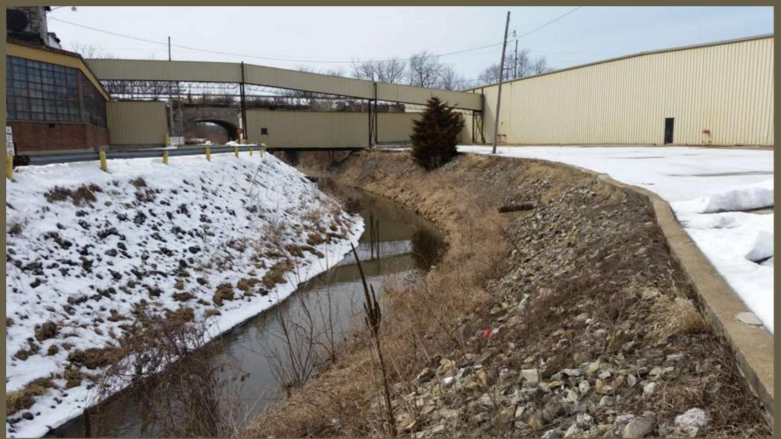
Looking downstream from the N. Patterson Street Bridge towards the RR Bridge. Parking lots on both sides of the channel come right to the top of bank. Notice that the box bridge in the background sits on the parking lot and would restrict any flood flows.
