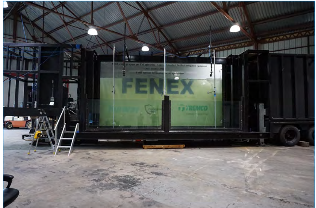
LOAD TEST OF 9' OF WATER ON 20' X 11' FLOOD WINDOW
