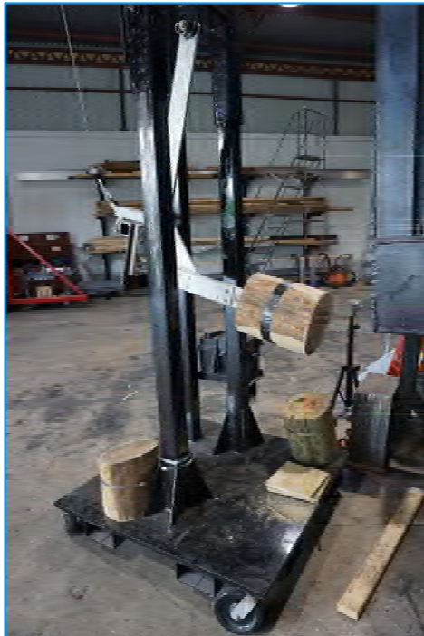
1,000 LB. IMPACT AT 8 FPS ASCE 7 REQUIREMENTS
